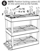
Flip unit upright after casters are securely installed.
